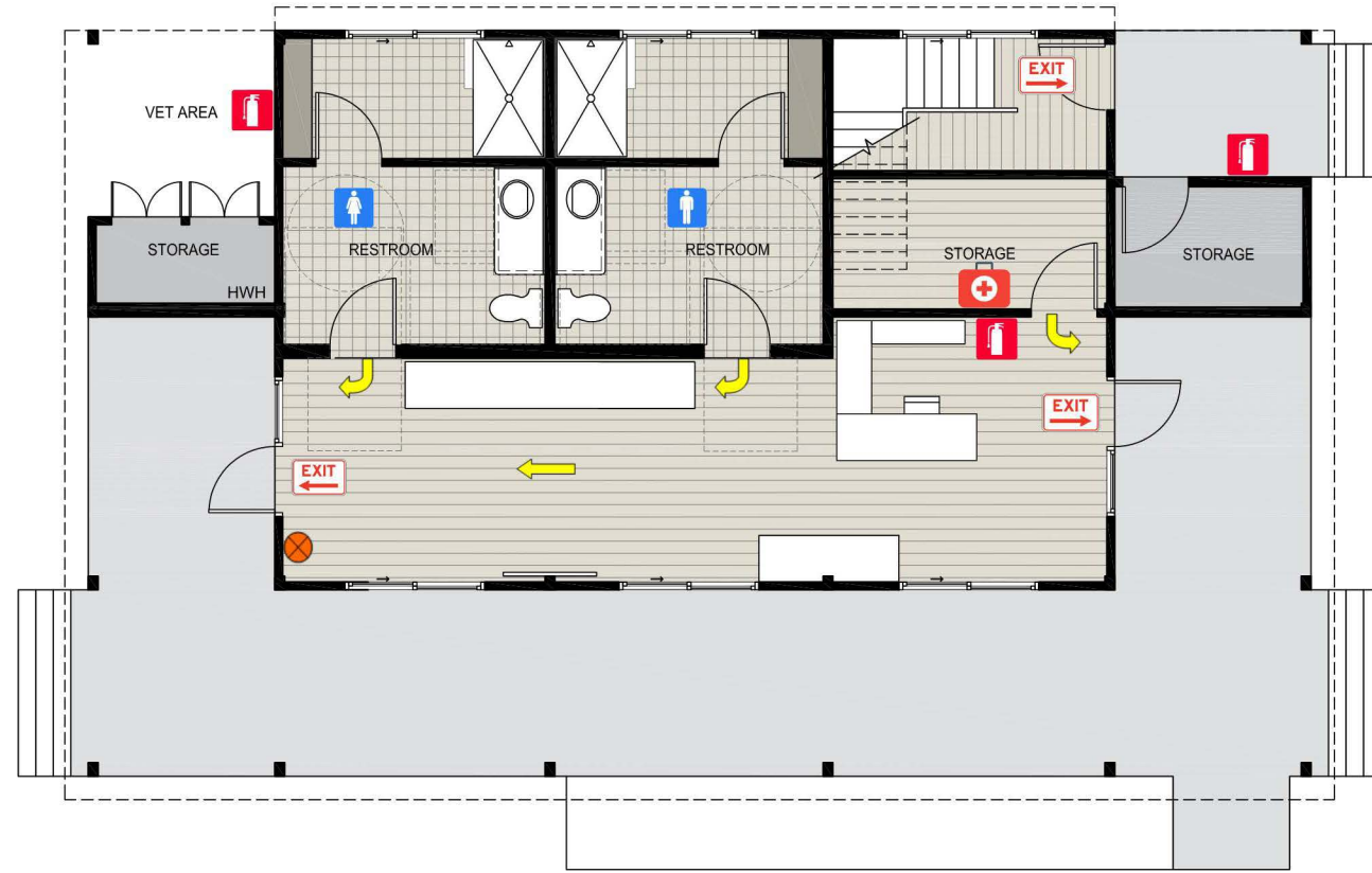
OFFICE TYPE II - LOWER FLOOR PLAN
