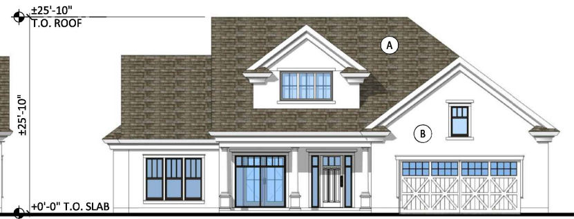
2 SECONDARY DWELLING UNIT FRONT ELEVATION SCALE: 1/8" = 1'-0"
