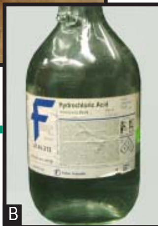
Figure 1: Anhydrous hydrogen chloride gas is stored as a liquid in pressurized containers [A]. Aqueous solutions of hydrogen chloride are called hydrochloric acid or muriatic acid [B] and are found in commercial chemical or swimming pool supply houses. Photos: Courtesy of CA Department of Justice.
