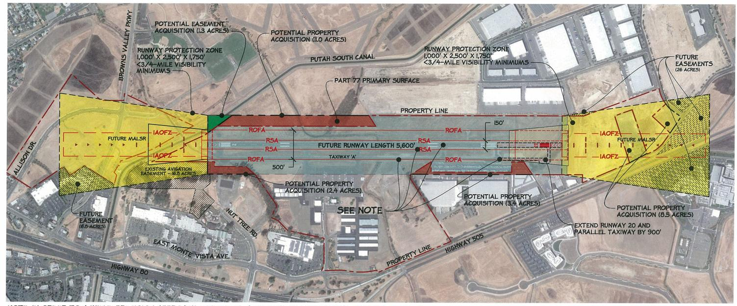
NOTE: IN ORDER TO ACHIEVE PRECISION APPROACH MINUMUMS, A NUMBER OF DIMENSIONAL CRITERIA CHANGES WOULD BE REQUIRED, INCLUDING AN INCREASE IN RUNWAY WIDTH FROM 75' TO 100', AN INCREASE IN RUNWAY/TAXIWAY SEPARATION FROM 240' TO 300', AN INCREASE IN RSA SIZE, AN INCREASE IN THE SIZE OF THE ROFA, AMONG OTHER THINGS. THESE DIMENSIONAL CRITERIA ARE NOT ILLUSTRATED ON THE EXISTING ALP.
